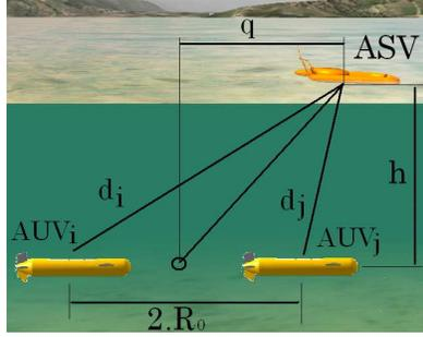
Fig. 4. A fleet of AUVs supervised by the ASV.  $h$ : operating depth,  $R_0$ : the radius of the circular formation, and  $q$ : the distance between the ASV and the projection of the center of formation on the surface.
