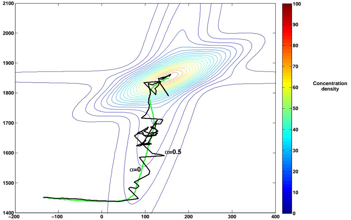
Fig. 5. The trajectory of the center of formation  $\mathbf{c}$  subject to random packet dropout and no repetition in coding (the black trajectory) and the trajectory of the center of formation  $\mathbf{c}$  in the absence of dropout (the green trajectory).
