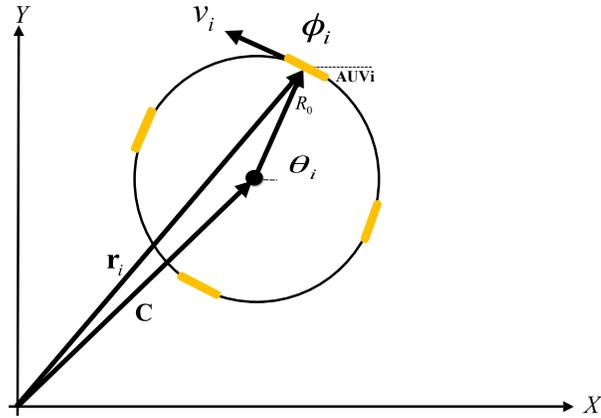
Fig. 2. A fleet of AUVs in a circular formation in the reference coordinate system.  $\theta_i$ : rotational angle,  $\phi_i$ : heading angle,  $v_i$ : forward velocity,  $c$ : the center of formation vector,  $r_i$ : position vector, and  $R_0$ : the radius of the circular formation.
