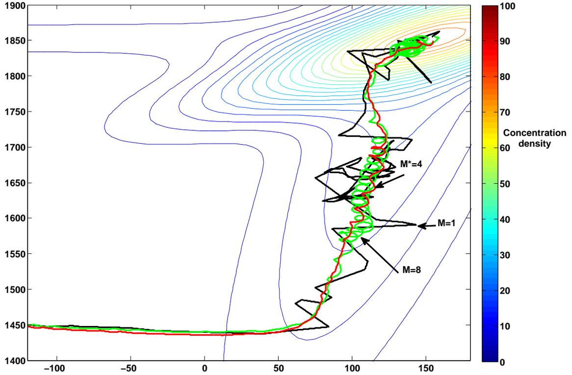
Fig. 7. The trajectories of the center of formation  $\mathbf{c}$  subject to 50 percent packet dropout in communication from AUVs to the ASV and 5 percent packet dropout in inter-AUV communication as well as in communication from the ASV to AUVs.
