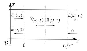
Figure 2: Illustration of the right-going and left-going propagating mode amplitudes  $\hat{a}(\omega, z)$  and  $\hat{b}(\omega, z)$ . The source generate the probing wave  $\hat{a}_0(\omega)$ , the reflected wave is  $\hat{b}(\omega, 0)$  and the transmitted wave, which is our interest is  $\hat{a}(\omega, L/\varepsilon^s)$ . Note that there is no energy coming from  $z > L/\varepsilon^s$ .
