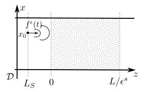
Figure 1: Illustration of the waveguide model. The source  $f^{\varepsilon}$  generates a wave that is propagating in the positive z direction. The section  $z \in [0, L/\varepsilon^s]$  is randomly heterogeneous with long range correlations. Our objective is to characterize the pulse as it emerges on the termination of the random section at  $z = L/\varepsilon^s$ .
