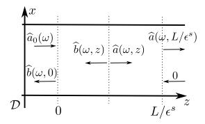
Figure 2: Illustration of the right-going and left-going propagating mode amplitudes  $\hat{a}(\omega, z)$  and  $\hat{b}(\omega, z)$ . The source generate the probing wave  $\hat{a}_0(\omega)$ , the reflected wave is  $\hat{b}(\omega, 0)$  and the transmitted wave, which is our interest is  $\hat{a}(\omega, L/\varepsilon^s)$ . Note that there is no energy coming from  $z > L/\varepsilon^s$ .
