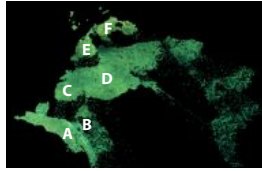
(b) Point cloud from 18 views in full size processed with the IGN software MicMac ( \simeq 85,000 points)
