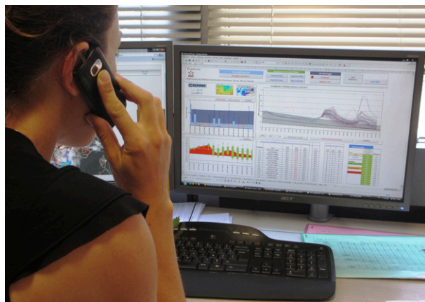
FIG. 2. Électricité de France operational river forecaster Audrey Valéry consults by phone with a dam manager about floods expected on the Drac River in southeastern France. On the screen are ensemble streamflow forecasts generated by a rainfall-runoff model. Preparing and running models are only two aspects of the forecasting process. Hydrologists also coordinate with the producers of other forecasts (e.g., meteorologists), review data, interpret model output, assess forecast confidence, consider nonmodeled factors (including anecdotal information), coordinate with water managers whose actions both depend on and affect river flow, translate model output into the decision-maker's context, and respond to user requests.
