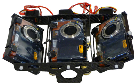
Figure 12b. The tri-camera system as built.
