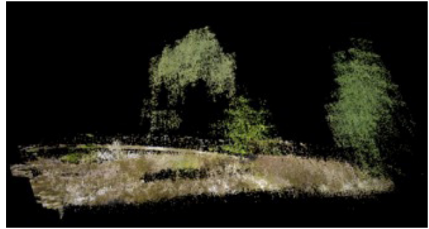
Figures 16a, 16b. Two views of the points cloud extracted from the stereo couple (source: Petitpas).
