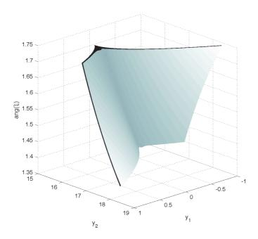
Fig. 2. Caustic surfaces  $\Xi(y,\xi)$  (dark gray) and  $\check{\Xi}(y,\xi)$  (light gray) of  $\Lambda$  and  $\check{\Lambda}$  corresponding to propagation through a low velocity lens (cf. section 5): The singular regions of  $\Lambda$  and  $\check{\Lambda}$  do not intersect.
