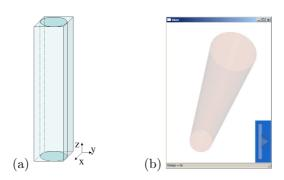
Figure 2: Geometry of riser reactor cylinder: (a) embedded into its square-base cylinder and (b) VTK rendering of the geometry boundary before starting the simulation.
