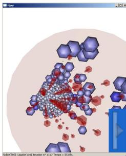
Figure 5: Yet another view from the top into the column. The online interactive visualization allows us to explore and travel into the flow. Solid catalyst particles and gas velocities represented par red arrows are plotted.
