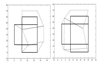
Figure 7 : Example of two optimised virtual fields (dotted line) used for identifying  $C_1$  and  $C_2$ . The virtually deformed fields are superimposed on the undeformed virtual mesh (solid line).
