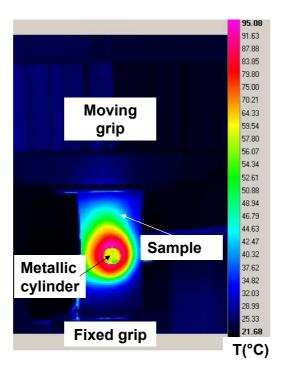
Fig. 3. Cartography of sample surface temperature
