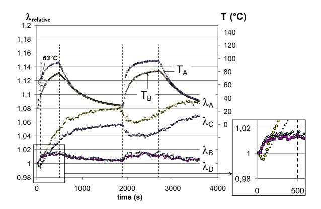
Fig. 5. Relative stretch ratio in zone A, B, C, and D, and temperature in zone A and B versus time
