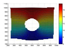
(a) displacement in the loading direction
