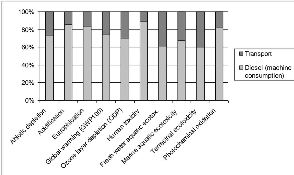
Figure 2: environmental impacts of the Brou demolition site
