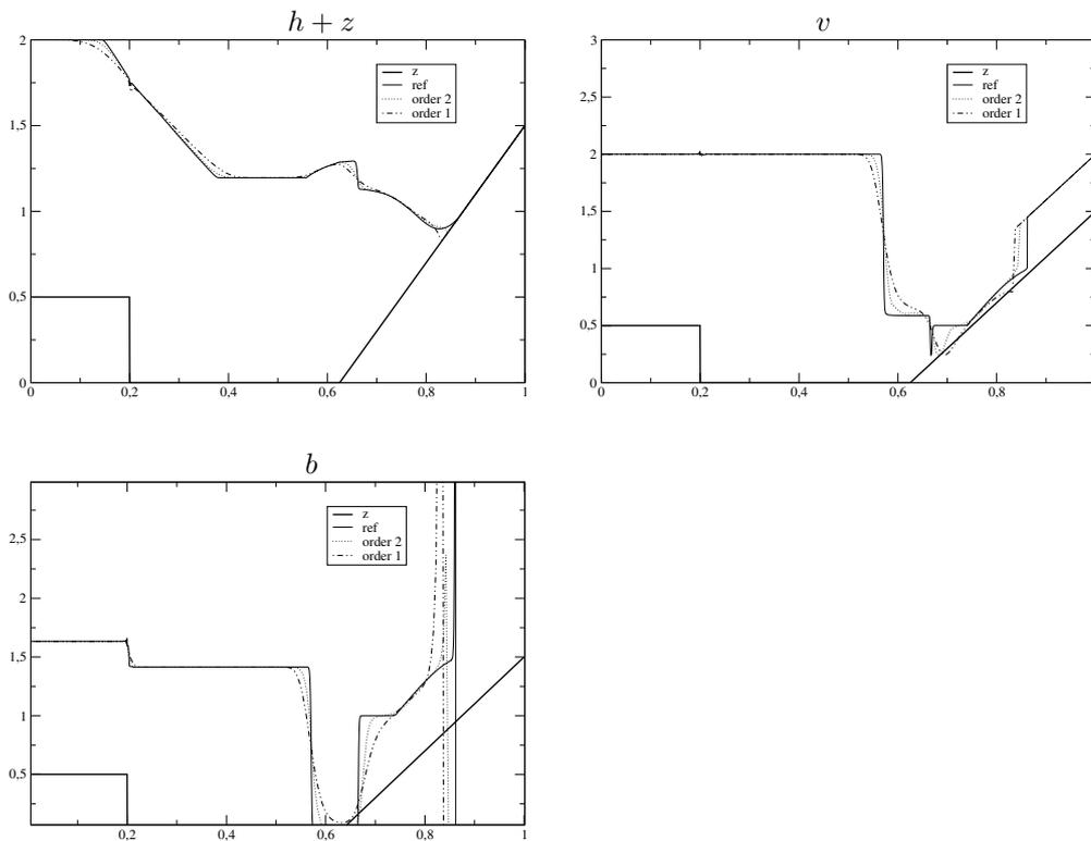
Figure 5: Components  $h+z$ ,  $v$ ,  $b$  at time  $t = 0.08$  computed at first and second order with 200 points with the first scheme of Theorem 3.1. The reference solution is the continuous line. The second scheme of Theorem 3.2 gives almost identical results (not shown).
