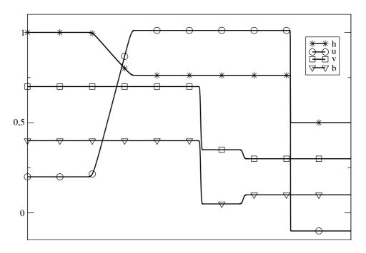
Figure 3: Riemann solution for Test 1 at time t=0.1 computed with the HLL flux or the 5-wave solver with 10000 points
