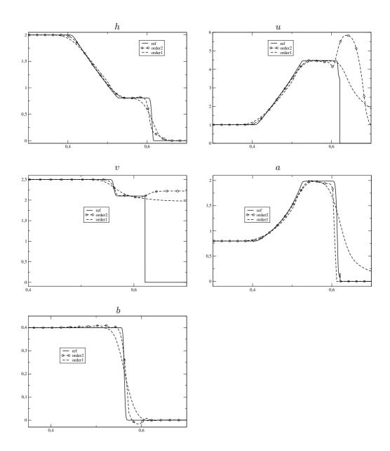
Figure 8: Components h, u, v, a, b for Test 3 at time t = 0.05 computed at first and second order with 200 points. The reference solution is the continuous line. The height h vanishes on the right state, leading to irrelevant values of u, v, a, b since only the conservative variables hu, hv, ha, hb make sense.
