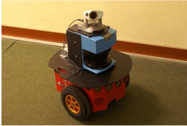
Fig. 5: The Pioneer 3 DX robot with its Canon VC-C50i camera.
