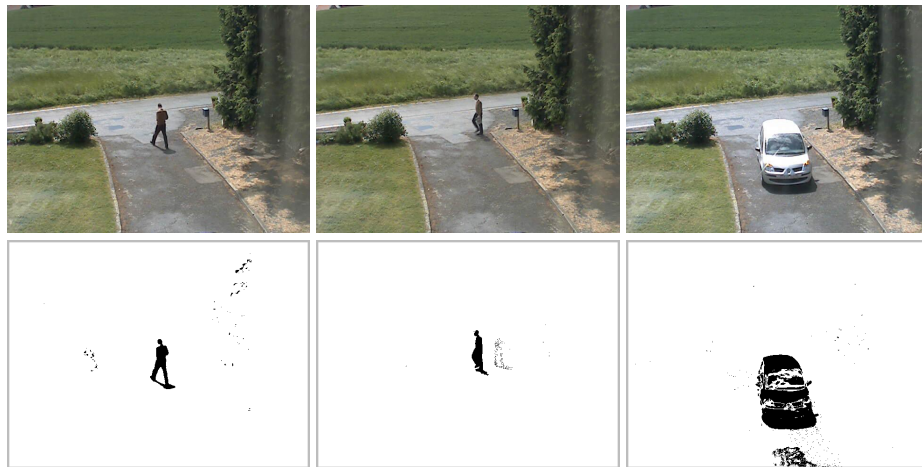
Fig. 19. Background subtraction based on sample and consensus using a codebook of colour local jet features.
