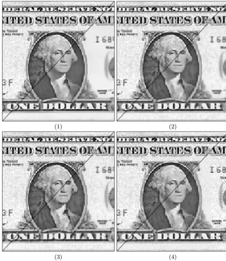
Fig. 15. NL-means filtering in the local jet feature space. (1) Limited range ( \mathcal{N}(\mathbf{x}) is a 17 \times 17 square neighbourhood of \mathbf{x} in the image domain). (2) Unlimited range, exact search ( \mathcal{W}(\hat{\mathbf{x}}_f) corresponds to the 30 NN in the local jet domain), (3) Unlimited range, approximate search ( \varepsilon = 10.0 ), (4) Unlimited range, exact search, with quantised feature space (1938 words in the dictionary).
