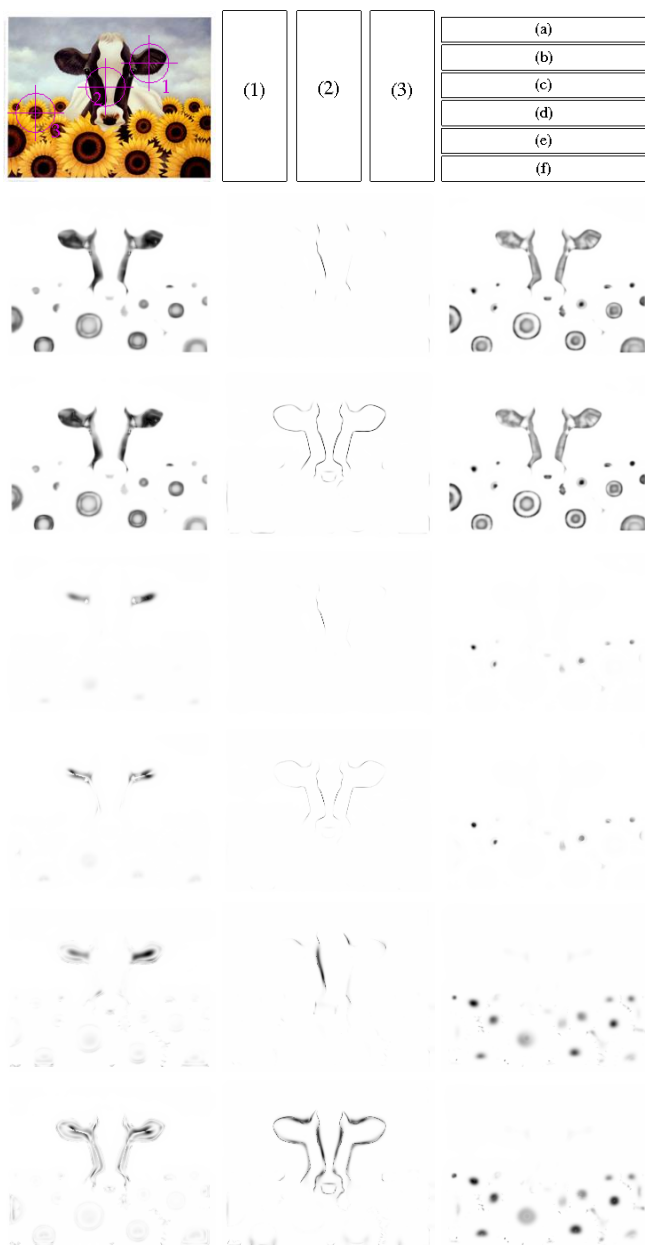
Fig. 8. Similarity maps for 3 different pixels: (1), (2) and (3), and 6 different distances: Single scale: (a) canonical components (CC), (b) rotation invariant components (RIC), Pan-scalic: (c) CC, (d) RIC, and Trans-scalic: (e) CC, (f) RIC. (Painting by Lowell Herrero)
