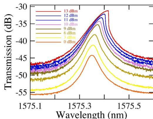
FIG. 4. Transmission of the resonance associated with a width-modulated waveguide cavity as a function of the pump power measured at the laser output. The  $Q_l$  factor at low excitation is 31 000. The number of supporting tethers is 16.
