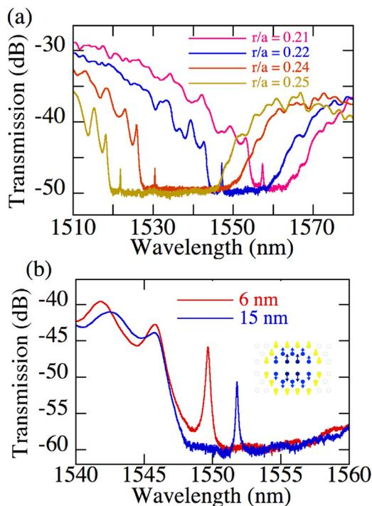
FIG. 3. (a) Transmission dependence as a function of  $\frac{r}{a}$  ratio. The maximum hole displacement for the cavity is 9 nm. The barrier coupling length is  $13a$ . The sample thickness is 330 nm. (b) Transmission dependence as a function of lateral displacement for the width-modulated waveguide cavity. The inset shows a schematics of the lateral hole displacements for the cavity. The blue and yellow arrows correspond to  $2/3$  and  $1/3$  of the main displacement.
