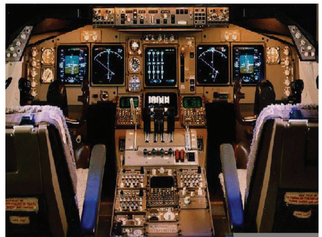
Fig. 4. Example of a computer-based, concentrated user interface—the glass cockpit (transition to glass cockpit for the Boeing 747).
