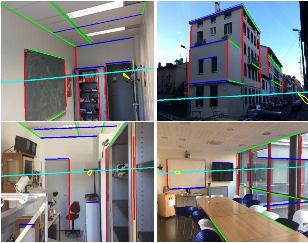
Figure 6: Some photos of the dataset with their ground truth line segments (red, green, blue), the horizon line computed from the IMU data (cyan line) and the polygon of the uncertainty region computed on the red line segments. On the top row, the horizon lines computed with the IMU data do not intersect the yellow polygons because of the bias of the IMU data.
