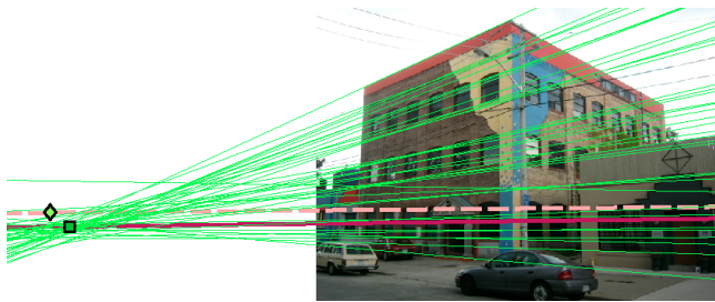
Figure 2: The green square is the estimated VP by [15] (associated horizon in red). The light green point (associated horizon dashed) is the VP after orthogonalization of the Manhattan directions: it lies far from the common intersection zone of the associated line segments.
