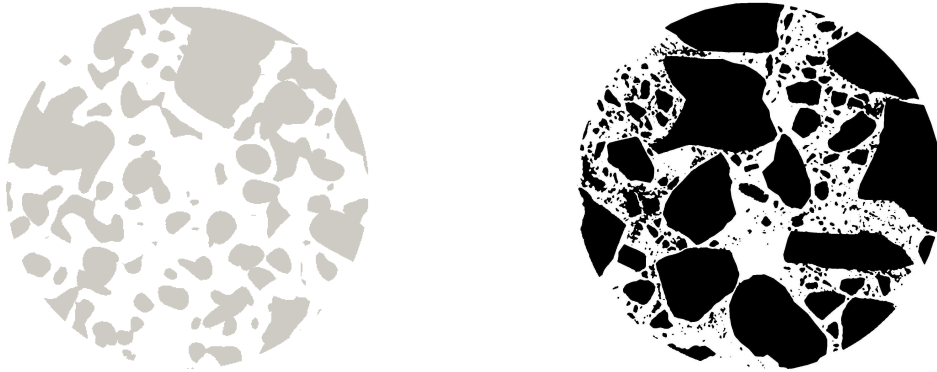
(a) Excursion set extracted from FIG. (16). (b) Segmented X-ray microtomography from Qier (2014).
