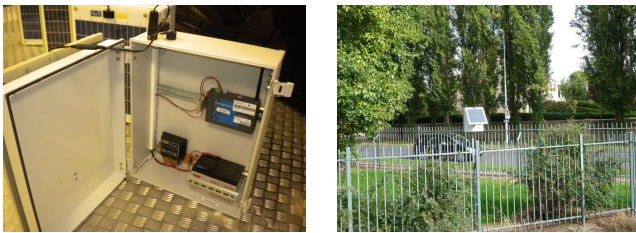
Fig. 2. An RSU built at UTC and used to exchange information with passing vehicles. The RSU-download application allows for instance to update maps.
