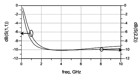
Figure 9 : SiGe LNA input and output matching
