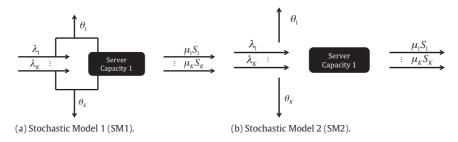
Fig. 1. Multi-class single-server queue with abandonments.
