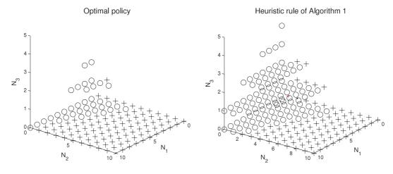
**Fig. 5.** Optimal policy and heuristic for a 3-class single server example for SM2. Circles indicate that class 1 is served, pluses that class 2 is served and absence of a sign corresponds to class 3 being served.
