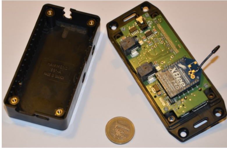
Fig. 3. Airbox – platform based on IGEP development boards, Xbee modem with external antenna is shown attached to the dedicated slot (1 euro coin is used for the comparison of sizes)
