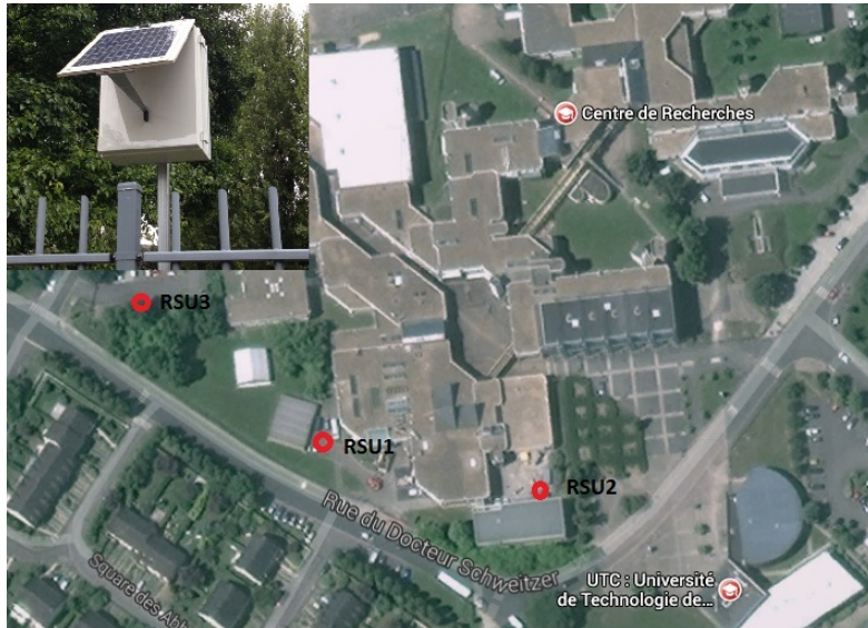
Fig. 4. Geographical position of the road-side units, RSU3 is shown in the upper left corner encased with an energy harvesting module
