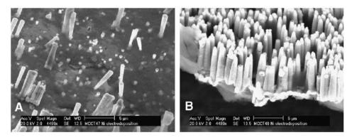
Fig. 6. Electrodeposited Ni conical nanowires (base diameter: 800 nm; top diameter: 100 nm; length 7  $\mu$ m) after dissolution of metallized track-etched PC membrane. PC films were irradiated with Pb of 0.63 MeV/amu. Etching conditions: Asymmetrical etching from the ion entry side of PC films using a two-cell compartment assembly: (A) 70 °C, 30 min, NaOH 2 N in the first compartment, no neutralizing solution in the last compartment; (B) 70 °C, 30 min, NaOH 2 N in the first compartment.
