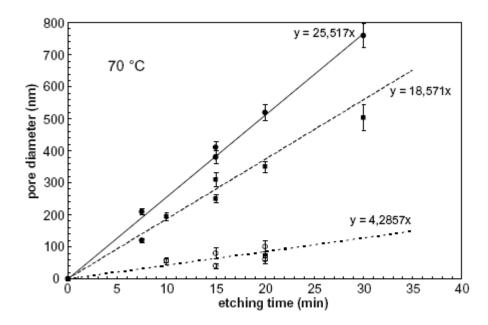
Fig. 2. Pore diameters estimated by SEM versus etching time. Etch conditions: 70 °C, NaOH 2 N.  $\blacksquare$  Exit face in contact with etch solution.  $\square$  Entry face in contact with water.  $\bullet$  Exit face in contact with water.  $\bullet$  Entry face in contact with etch solution.
