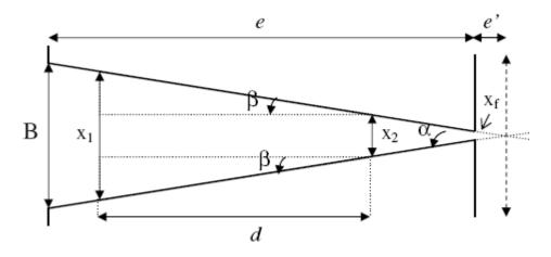
Scheme 1. Geometry of conical pore.
