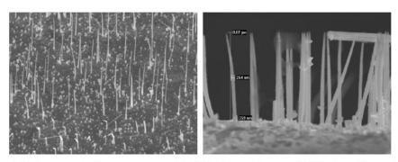
Fig. 7. PC matrix irradiated with low-energy ion beam: entry energy of 0.633 Mev/amu – exit energy of 0.1 Mev/amu. Fluence: 1e8 ions/cm<sup>2</sup>. Asymmetric etching: 0.1 MeV/amu etched face, 70 °C, NaOH 2 N, 15 min. Ni electrodeposition. PC matrix is dissolved. Ni nanowires track replica:  $X_f = 17$  nm,  $\alpha = 2.3^{\circ}$ .
