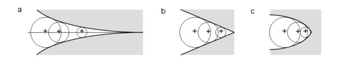
Fig. 5 Typical etch figures for (a) increasing, (b) constant and (c) decreasing etch-rate. The crosses mark the center of the spherical "waves" emitted at equal time intervals [15]
