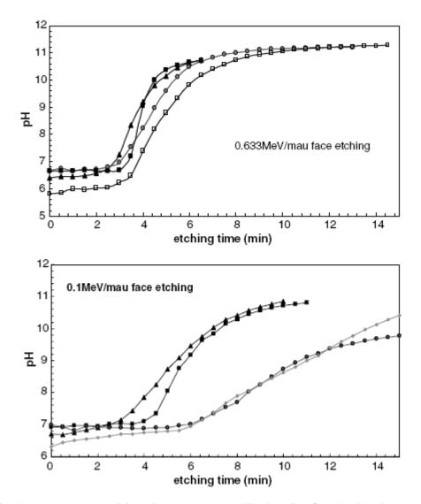
Fig. 3. pH versus etching time curves at ( $\Box$ ) 65 °C, ( $\bullet$ ) 70 °C, ( $\blacktriangle$ ) 75 °C and ( $\blacksquare$ ) 80 °C.
