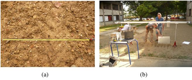
**Fig. 1:** (a) Surface roughness  $SRF$  measurements; (b) Synchronous samplings using laser and chain.
