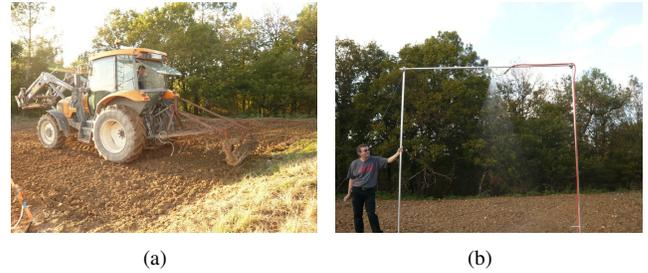
**Fig. 2:** Different (a) surface roughness; (b) soil moisture setting up in GB-SAR experiments.
