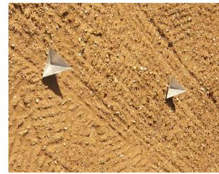
Fig. 8: The trihedral corner reflectors within scene
