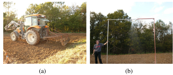
Figure 4: Different (a) surface roughness; (b) soil moisture setting up in GB-SAR experiments.
