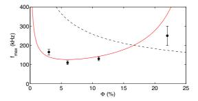
FIG. 2: Frequency of the maximum of attenuation as a function of the liquid fraction, for median radii of 40  $\mu$ m. Dashed line is the Minnaert resonance frequency with an effective density:  $f_M/\sqrt{\Phi}$ . Solid line is the prediction of our model.
