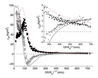
FIG. 5: Comparison between the measured effective complex density (o real part, • imaginary part) and prediction of the equivalent of Eq. (2) in the polydisperse model (see SM1).
