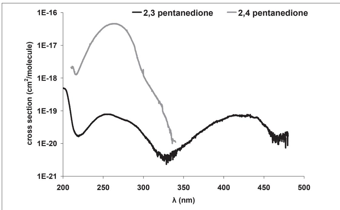
Figure 1. UV spectra obtained at 298 K for the two studied compounds.
