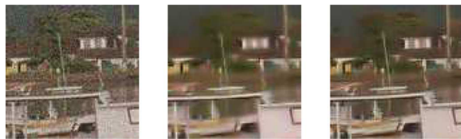
Fig. 12. Zoom the test images. Left: Original image with additive Gaussian noise. The SNR is equal to 15 dB. Middle: Wavelet-based denoising in the RGB space. Right: Wavelet-based denoising in the curvelet-GMCA space.
