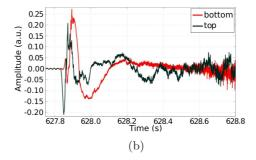
Figure 1: Typical temporal signal of acoustic emission at a precursor (a) and at an avalanche (b) recorded by two hydrophones buried at half depth in the bulk of the layer. One is placed in the upstream part of the packing when flowing and the second is placed in the downstream part of the packing.
