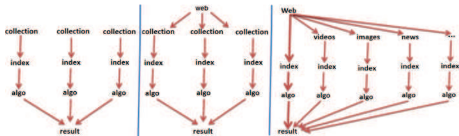
Fig. 3. Simple schemas for federated search (left), metasearch (center), and cross-vertical aggregated search (right).
