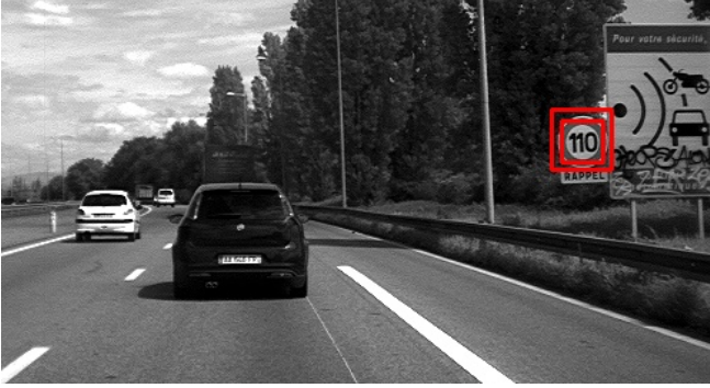
Fig. 3. Multiple detection case. When the signs are close to the camera, the template-matching algorithm can detect two circles (the inner and the outer circle) for the same sign leading finally to a set \Theta_{Y_j} of 2 detected objects.
