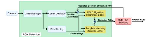
Fig. 3. Block-diagram of the ROI detector.
