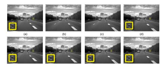
Fig. 8. Impact of the candidate position prediction feedback in 4 successive frames. (Top) Without feedback. (Bottom) With feedback.
