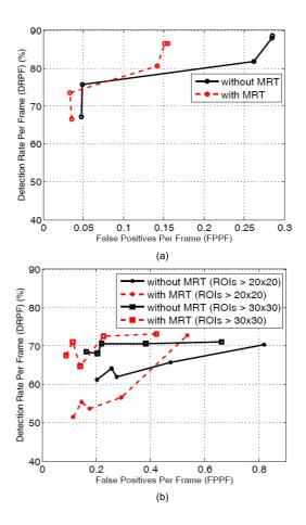
Fig. 9. Receiver Operating Characteristic (ROC) curves without and with MRT for circular (a) and triangular (b) signs.
