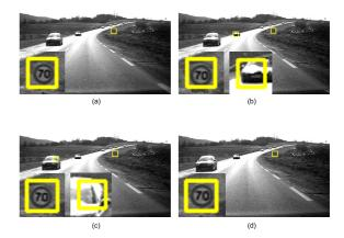
Fig. 7. Detection results without MRT in successive frames. (a) and (d) Correct sign detection. (b) and (c) Presence of false positives.
