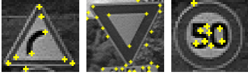
Fig. 4. Examples of detected corners related to traffic signs.
