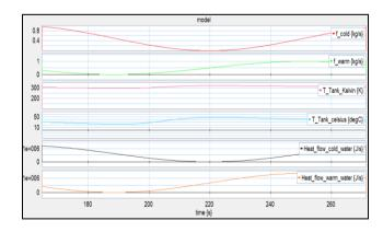
Figure 8. Water temperature variation inside the tank according to the variable water mass flows.
