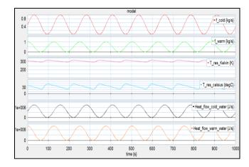
Figure 7. Simulation results of the bond graph model for variable mass flows.
