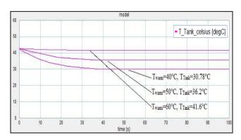
Figure 6. Influence of the warm water's temperature on the water temperature inside the tank.
