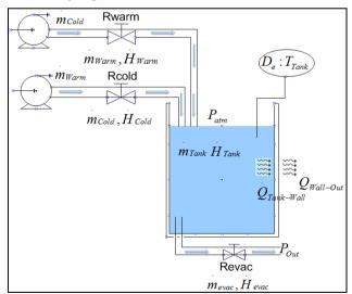
Figure 1. Synoptic scheme of the thermo-hydraulic system.
