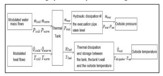
Figure 2. Word bond graph model of the thermo-hydraulic system.
