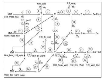
Figure 3. Pseudo bond graph model of the thermo-hydraulic system.
