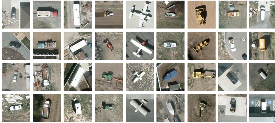
Figure 6: Images illustrating the different categories of the dataset. From left to right : car, truck, camping car, tractor, plane, boat, other, pickup and van.
