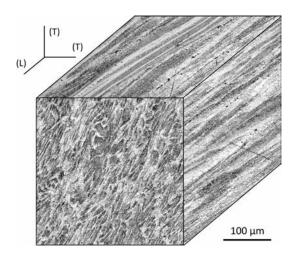
Fig. 1—3D reconstruction from optical micrographs of the grain structure of the base metal.
