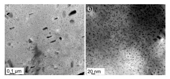
Fig. 5—TEM micrographs of the base metal in the T652 temper.
