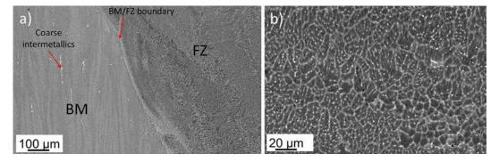
Fig. 4—SEM-BSE micrographs (a) of the weld-based metal interface and (b) of the weld nugget.
