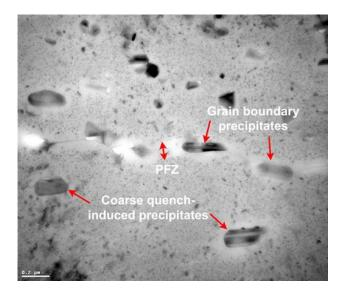
Fig. 6—Typical TEM micrograph of the base metal in the T652 + 48 h at 150  $^{\circ}$ C state.
