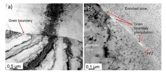
Fig. 7—TEM micrographs of the fusion zones (a) in the NA state and (b) in the AA state.
