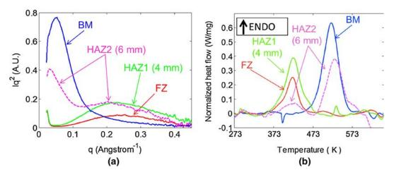
Fig. 11—SAXS Kratky plots (a) and DSC thermograms (b) for different zones of the weld (NA state).
