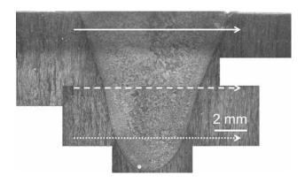
Fig. 2—Optical micrograph of the weld—dark field mode.
