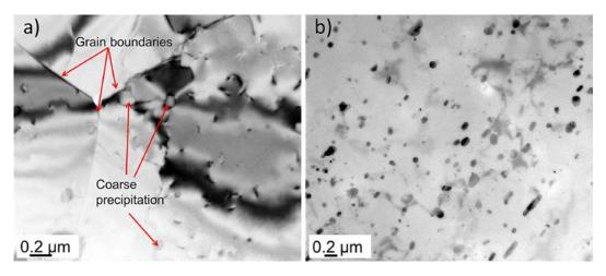
Fig. 9—TEM micrographs in the heat-affected zone (a) 5 mm from the center of the fusion zone and (b) 6 mm from the center of the fusion zone (NA state).
