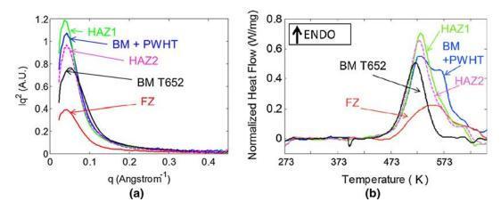
Fig. 12—DSC thermograms for different zones of the weld (AA state).
