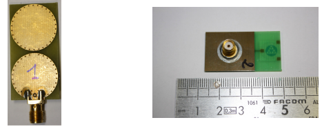
Fig. 8. Thomson 1 (left), fractal structure (right) antennas
