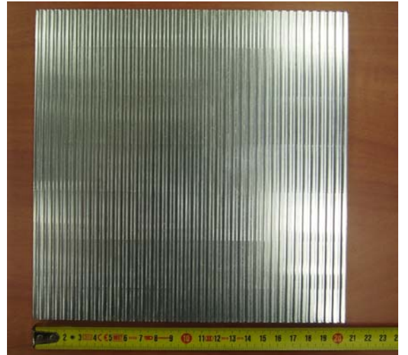
Fig. 9. A larger 80-groove array whose size is 200mm \times 200mm
