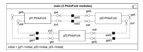
Figure 4. A model for the dinner of 3 philosophers. The composite type declaration contains three instances and six private synchronizations. For instance, private synchronization *eat*<sub>2</sub> synchronizes *pf2.eat* and *pf1.put*.
