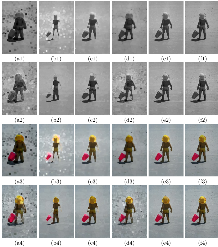
Fig. 6. Comparison of the conventional gray-scale (row 1) and the conventional RGB component-wise ordering (row 3) morphological operations, with respect to the proposed BPT-based spatial-spectral \pi -ordering (rows 2 and 4) obtained using a square 11 \times 11 structural element: (a) erosion, (b) dilation, (c) closing, (d) opening, (e) closing by reconstruction, and (f) opening by reconstruction.
