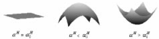
Fig. 4. Illustration of Hölder exponent \alpha^H for different spatial variations of intensity. Knowing the value \alpha_0^H for an homogeneous region, we have \alpha^H > \alpha_0^H for a concave region and \alpha^H < \alpha_0^H for a convex region.
