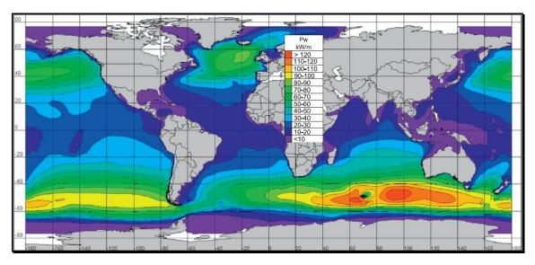
Fig. 2. Global annual mean wave power estimation in kW/m spanning 10 years period [6].
