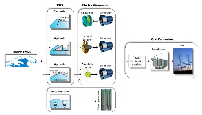
Fig. 7. WEC different type of conversions.
