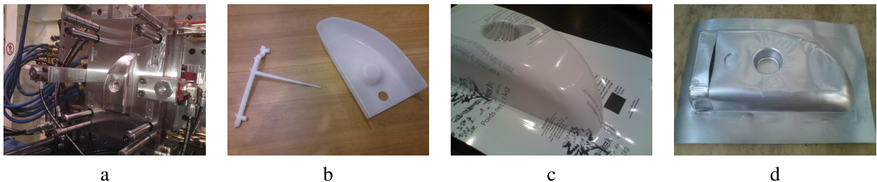
Figure 2 : Industrial context. The hydraulic press and the kernel of the mold (a). The resulting object after injection (b). Thermoformage (c). Insert Molding (d).
