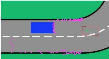
Fig. 3. Obstacles represented in world frame  $\{W\}$  (in blue), with detection of obstacles and also navigable zone boundaries (in pink).
