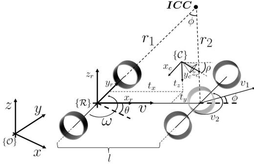
Fig. 1. Cinematic model diagram for a front wheel car-like robot. In this model the vehicle reference frame  $\mathcal{R}$  performs circular trajectories related to the instantaneous center of curvature (ICC). The pinhole camera frame is also represented in  $\mathcal{C}$ .
