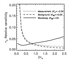
**Figure 1.** Relative sensitivity of absorption optical depth  $\tau_a$  to variations of measured (dotted), background (dashed), and blackbody (solid) brightness temperatures  $dT_m = -0.3 \text{ K}$ ,  $dT_{BG} = 0.5 \text{ K}$ , and  $dT_{BB} = 2 \text{ K}$ , respectively.
