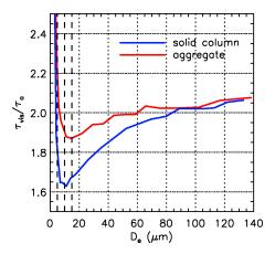
**Figure 2.** Simulations of the ratio between CALIOP optical depth at  $532\,\mathrm{nm}$  ( $\tau_{\mathrm{vis}}$ ) and IIR absorption optical depth at  $12.05\,\mathrm{\mu m}$  ( $\tau_{\mathrm{a}}$ ) at  $\tau_{\mathrm{a}}=0.25$  against effective diameter  $D_{\mathrm{e}}$  for hexagonal solid columns (blue) and aggregates (red). Vertical dashed lines indicate  $D_{\mathrm{e}}$  smaller than  $15\,\mathrm{\mu m}$  (see text).
