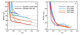
**Figure 6.** (a) Median  $\tau_{\rm vis}/\tau_{\rm a}$  ratio and (b) standard deviation from standard CALIOP constrained retrievals (thin lines) and from extended CALIOP optical depth measurements (thick lines) for type 1 clouds retrieved from measured  $R_{\rm BG}$  after correction for cloud radiative temperature. The vertical dotted lines highlight the differences for  $2\tau_{\rm a}$  between 0.3 and 0.6 (see text). Same data set and color code as in Fig. 5.
