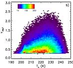
**Figure 11.** Two-dimensional histogram of (a)  $\tau_{\rm vis}$  ( $\eta=0.6$ ) and (b)  $\tau_{\rm vis,T}$  ( $\eta_{\rm T}$  from this study), and centroid temperature  $T_{\rm c}$ . The color code is the number of samples. Same data set as in Fig. 9.
