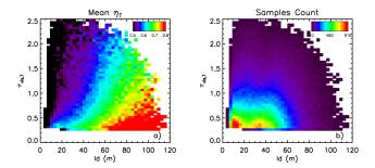
**Figure 10.** (a) Mean value of the multiple scattering factor  $\eta_T$  as a function of visible optical depth  $(\tau_{\text{vis},T})$  and estimated lateral displacement (ld); (b) associated number of samples. Same data set as in Fig. 9.
