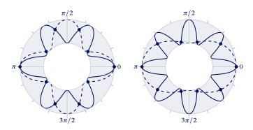
(a) waves  $cos(6\theta)$  and  $cos(4\theta)$  (b) waves  $cos(8\theta)$  and  $cos(2\theta)$ Figure 12. Aliasing effect: continuous external forcing waves and its corresponding sampled counterpart  $\bullet$  acting on the blades
