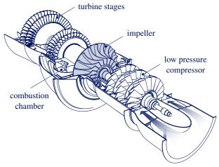
Figure 1. Cut view of an aeronautical engine
