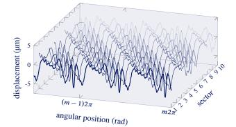
**Figure 10.** Steady-state response of the ten sectors: main blade leading edge radial displacement (the angular position of the bladed disk is used instead of time for the sake of clarity)
