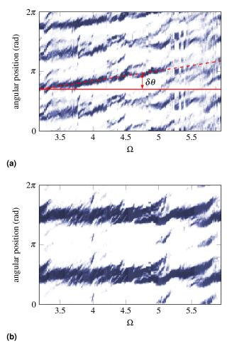
**Figure 24.** Contact areas maps. Line (- - -) illustrates the angular shift of the contact location with  $\Omega$ , (a) leading edge, (b) trailing edge
