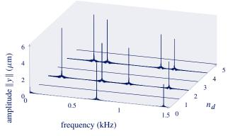
Figure 17. 2D Fourier transform of the radial contact force
