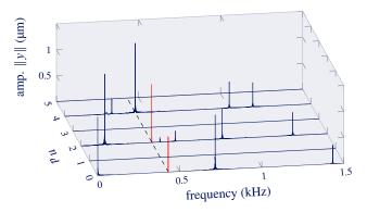
**Figure 11.** Two-dimensional Fourier transform of the impeller response. Red peaks on nodal diameters 0 and 2 along the dashed line are fictitious and added to illustrate the frequency clustering phenomenon
