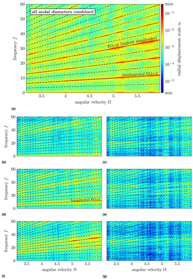
Figure 22. Interaction maps for a 2-lobe casing distortion, (a) interaction map, (b)  $n_d = 0$ , (c)  $n_d = 1$ , (d)  $n_d = 2$ , (e)  $n_d = 3$ , (f)  $n_d = 4$ , (g)  $n_d = 5$
