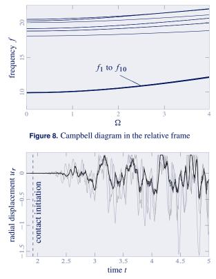
**Figure 9.** Convergence plot of the radial displacement:  $\eta = 50$  (—),  $\eta = 100$  (—),  $\eta = 150$  (—),  $\eta = 200$  (—), and  $\eta = 250$  (—)
