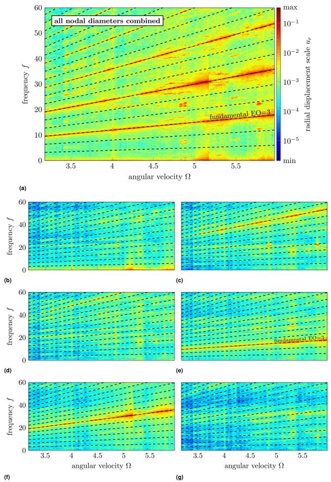
Figure 27. Interaction maps for a 3-lobe casing distortion, (a) interaction map, (b)  $n_d = 0$ , (c)  $n_d = 1$ , (d)  $n_d = 2$ , (e)  $n_d = 3$ , (f)  $n_d = 4$ , (g)  $n_d = 5$
