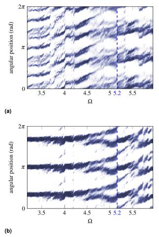
Figure 28. Contact areas maps, (a) leading edge, (b) trailing edge
