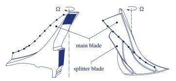
Figure 3. Elementary sector of the impeller
