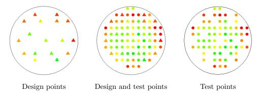
Figure 4: Color representation of thickness values. The 81 measurement locations are shown in the middle, including 17 design points (triangles, left) and 64 test points (bullets, right).
